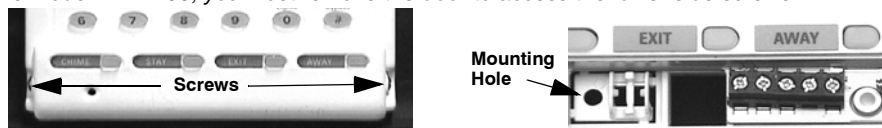
Figure 3. Removing Lower Cover to Access Lower Mounting Hole
